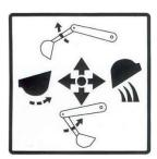
Push the right hand outer control lever, arm(dipper stick) moves away from operator, and pull back the lever, arm(dipper stick) moves toward the operator.
