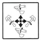
Push the left hand outer control lever, boom moves down, and pull back the lever, boom moves up. Also, pushing the lever fully forward into the detent position, allows the boom to float. In the float position, the boom can drift up or down without pressure.
